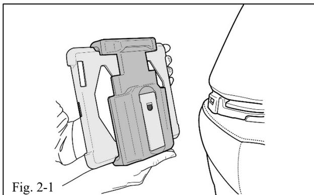
(a) To install the Holder, with or without a tablet mounted, open the arm at the back and insert it into the Combo Hook Dock (Fig. 2-1 & Fig. 2-2).
