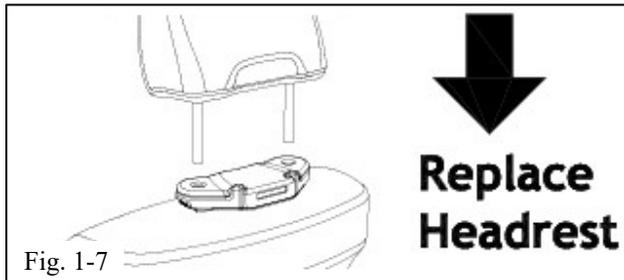
(i) Replace the head rest (Fig. 1-7). It should click when properly fitted.
