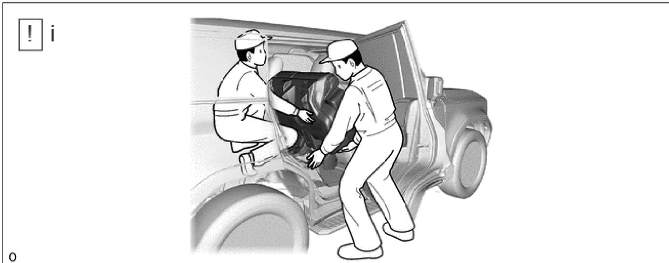
(1) Remove and carry the rear No. 1 seat assembly RH out of the vehicle.
