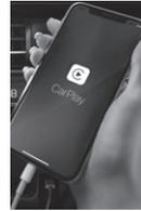
**STEP 2** Plug a compatible iPhone® into the USB media port using an Apple® approved cable or have the smartphone and vehicle connected through Bluetooth®.
