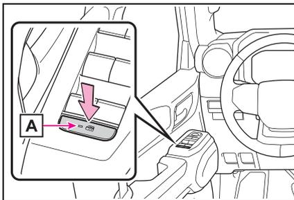
**■ The window lock switch can be operated when**
