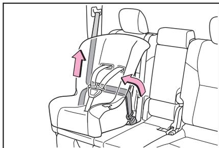
7 If the child restraint has a top tether strap, follow the child restraint manufacturer's operation manual regarding the installation, using the top tether strap to latch onto the top tether strap anchor. (→P.62)
