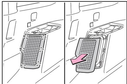
Disengage the 6 claws of the cover and remove the cover.
