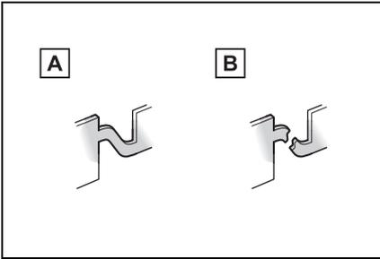
**A** Normal fuse**B** Blown fuse**■ After a fuse is replaced**
