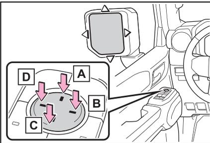
**A** Up**B** Right**C** Down**D** Left■ **Mirror angle can be adjusted when**
