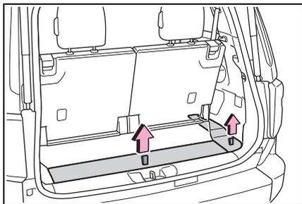
■ When installing the deck board (vehicles without third seats [rear of the luggage compartment] and vehicles with third seats)
