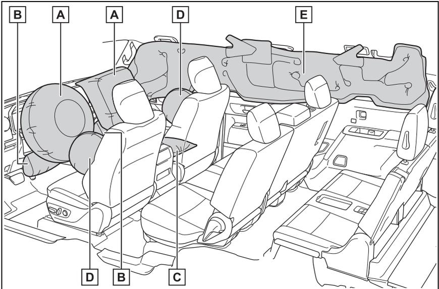
**A** SRS driver airbag/front passenger airbag
