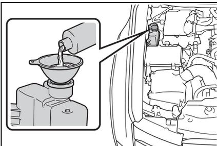
**6** Start the hybrid system and turn the air conditioning system on to check that the radi-
