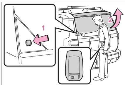
1 While carrying the electronic key, press the button to pop up the glass hatch.
