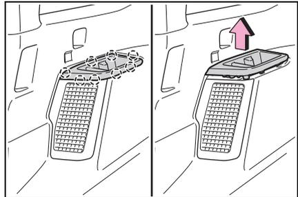
Disengage the 8 claws of the trim part and remove the trim part.
