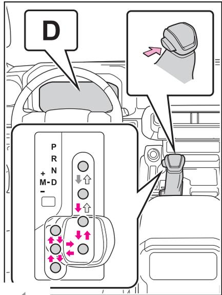
While the power switch is in the ON position and the brake pedal depressed\*, shift the shift lever while pushing the shift release button on the shift knob.
