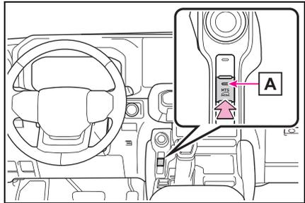
**2** Select the driving modes on the multi-information display while turning the MODE SELECT switch left and right.
