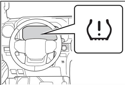
9 If the specified tire inflation pressure of the wheel set installed differs from that of the previous set, it will be necessary to perform the tire inflation pressure setting pro-
