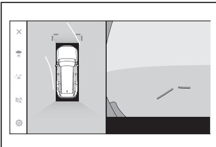
Displays course lines that are linked to operation of the steering wheel. (Yellow) These lines are displayed when the steering wheel is turned more than 90 degrees from the straight position.
